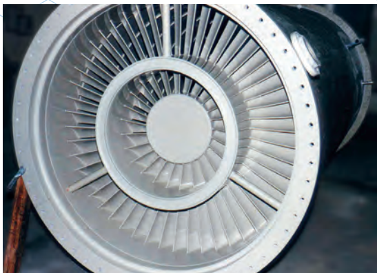
Swirl generator tube in a tube in the workshop
