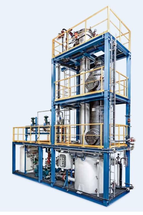
Vent gas treating system (VGTS) for the continuous renewable reformer (CCR) process, based on the UOP process
