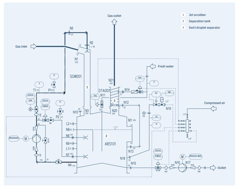
Flow diagram of a single-stage jet scrubber
