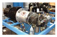
Maintenance-free sealing of proportioning pumps for polyde and isocyanate in high-pressure reaction casting machines
